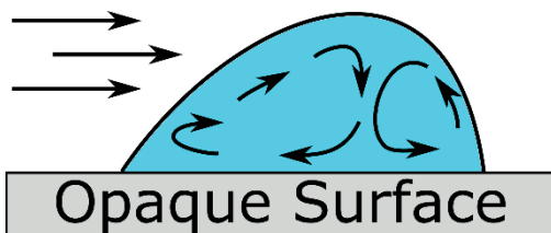
Fig. 1: Droplet in shear flow on an opaque surface. The only optical access is the oscillating phase boundary.
