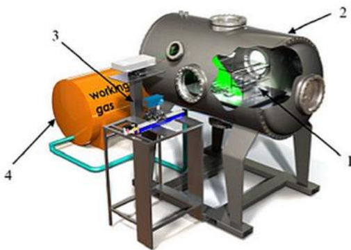
Fig. 3 Schematic of the SCALEX facility (left) and photograph of the experimental setup (right), with: (1) the generic passenger cabin, (2) pressure vessel, (3) sCMOS cameras, (4) working gas supply, (5) heat exchanger, (6) particle generator, (7) laser light sheet optics.
